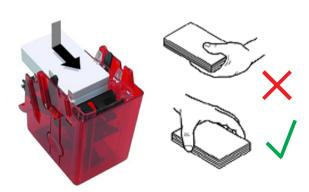
Turn the feeder over and insert the cards as shown. Ensure you handle the cards correctly.
