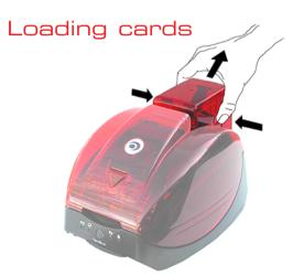
Remove the card feeder by pressing the side buttons.
