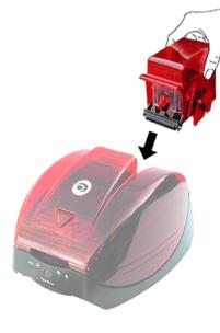
Place the feeder back into the printer until you hear an audible 'click'.
